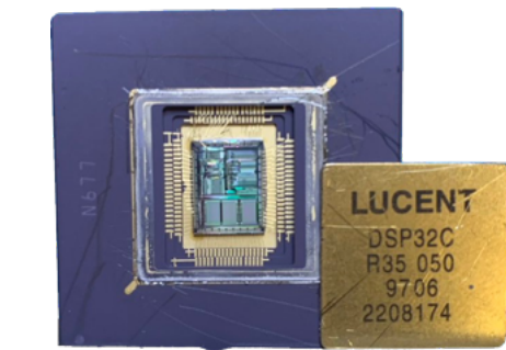
AT&T DSP-32C capable of 125m floating point multiply-accumulate operations/sec
